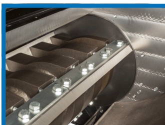
Rotor equipped with rotating end disks
